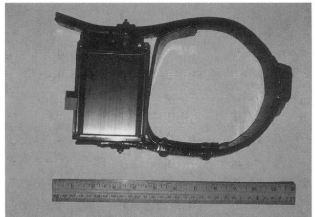
Fig. 1. Global Positioning System (GPS) radiocollar tested on wolves and white-tailed deer. Molded plastic box is 8.2 x 11.9 x 5.4 cm; the entire collar weighs 920 g.
